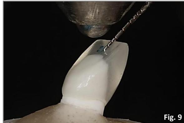
**(Figure 9)** Cemented crown (group S) embedded in resin and mounted in the universal testing machine. The load was applied 2.0-2.5 mm below the incisal edge.
