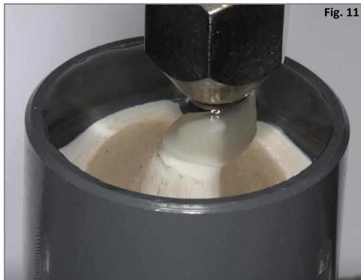
**(Figure 10+11)** Specimen mounted in the mechanical testing machine. The picture in Fig.10 is obtained from the side. Fig.11 shows a close-up from a top-side view. The basin provided the presence of water during fatigue testing. The holder guaranteed the immobility of the specimen. As the water basin is filled with water, the crown is hardly visible in Fig.10.
