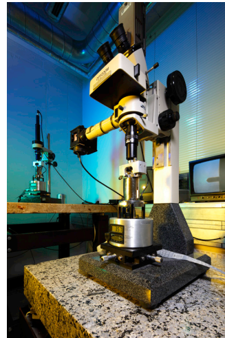
MultiMode AFM Nanoscope IIIa, Veeco
