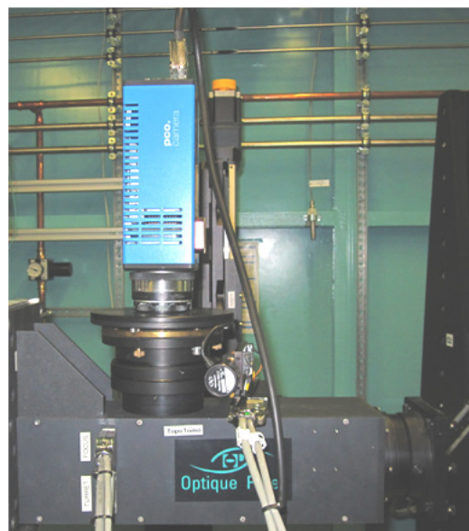
Fig. 3: The high resolution x-ray imaging setup at the ANKA – Topo Tomo beamline, Karlsruhe.
