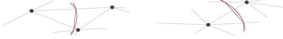
Figure 6.8: Two types of errors that may be introduced during re-initialisation. The red line represents the true \phi_0 . In blue are the segments that are found by the contour plotting utility. The segments intersect the mesh elements and are computed by a linear interpolation between nodal values. Left: Even if the intersection points are found with sufficient precision, the blue segment does not capture the true \phi_0 due to the segment's linear nature. Right: In this case the intersection is not found correctly.
