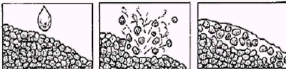
**Fig. 5-1:** Soil particles and aggregates that have been detached by raindrops are transported down the slope by runoff (TORRI and BORSELLI, 2000 in CHMELOVÁ and SARAPATKA, 2002).
