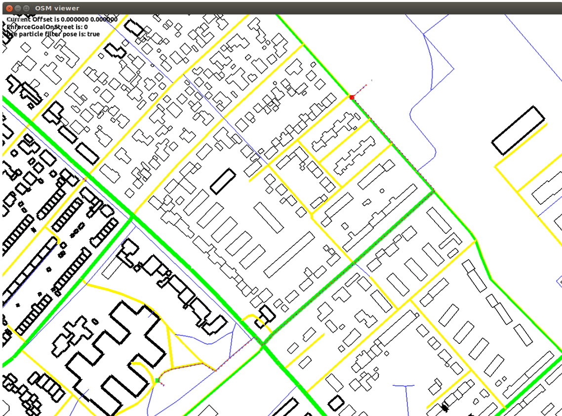
Figure 3.3: A screenshot of the GUI of our A* path planner on the road network. The GUI shows the planned path in gray from the robot on the top right to a goal on the bottom left. Both positions are not on the road network and are therefore first projected onto it (red and green squares).
