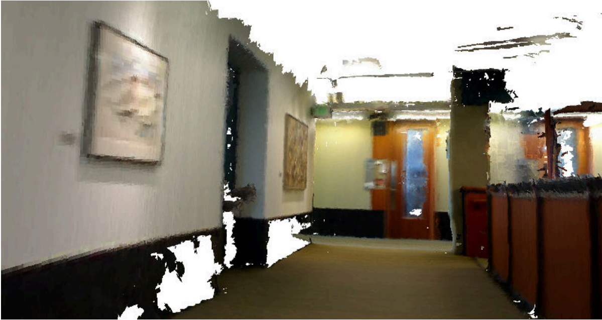
Figure 5.1: This picture illustrates the quality of a model built with our method at a resolution of 2 cm. We represent the surface with patches of size 20 \times 20 cm and encode each patch with a sparse code of an overcomplete dictionary. Generated from a 3.35 GB dataset, the resulting file size is 10.2 MB. For comparison, a colored occupancy Octomap of the same dataset has a size of 44.5 MB.
