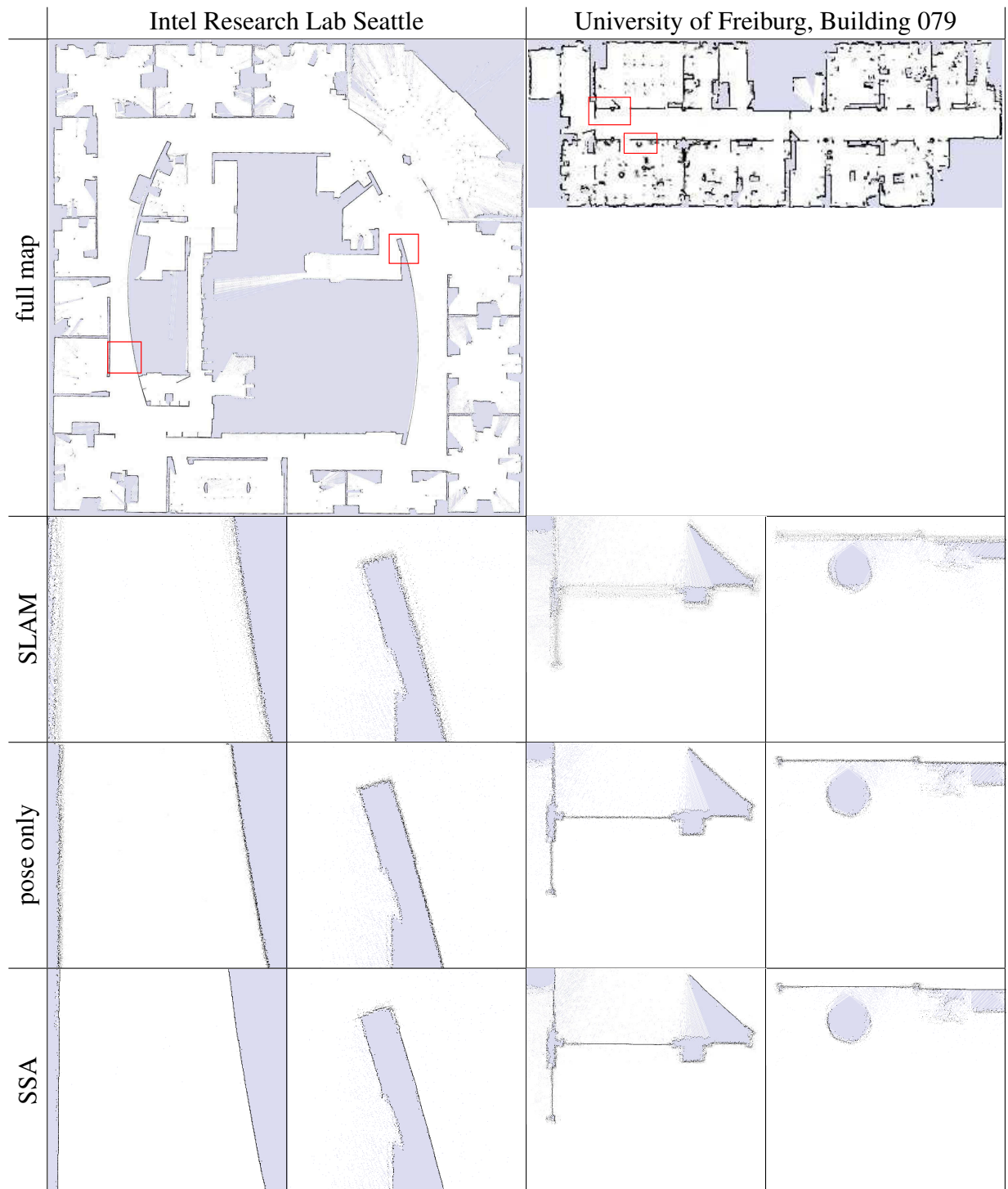
Figure 3.14: The top row of this figure shows the resulting maps for Intel and Freiburg 79 datasets. We enlarged some regions to visualize the differences in the SLAM results used as input (second row), the pose-only optimized result (third row), and the output of our method (bottom row). The bottom row shows only few blur and sharp borders between free and occupied cells.
