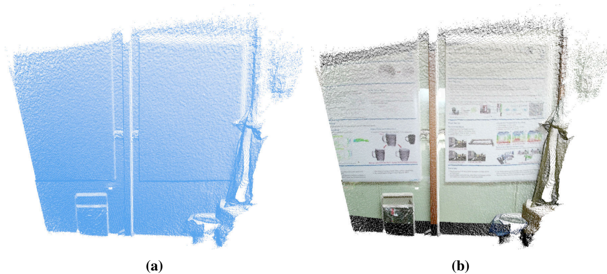
Figure 2.1: Example of a point cloud and a corresponding point cloud with color information.
