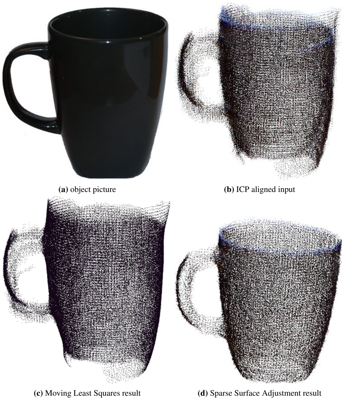
Figure 3.22: This figure illustrates differences between Sparse Surface Adjustment and Moving Least Squares. Therefore we acquired multiple scans of the cup shown in (a). Picture (b) shows the point clouds registered by using ICP and (c) illustrates the effect of MLS on the input data. Whereas the model looks smoother than the input it shows inconsistencies arising from errors in the estimate of the initial positions of the sensor. The picture in (d) depicts the results obtained by our approach on the same input data. The result appears to be more consistent.
