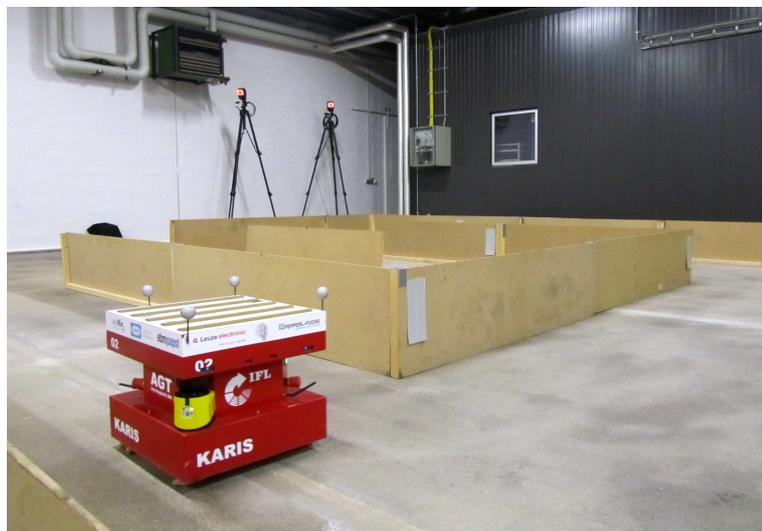
**Figure 6.7:** The holonomic KARIS robot operating in its experimental environment. It is equipped with two laser range finders mounted on opposite sides of the base for a 360° field of view. They detect reflective markers, which are attached to the walls, and are used as landmarks for localization. The reference positions of the robot are obtained by a motion capture system, part of which is shown in the back.
