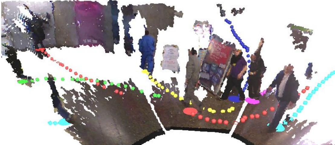
Figure 9.14: Visualization of the 3D point cloud produced by the three MS Kinect sensors including the positions and trajectories of eight of 31 tracks in the data set. The colored disks mark the current Kalman filter estimates of the target positions, the small dots show their past trajectories. The tracker maintains full 3D estimates as it can be seen by the dark blue trajectory of the subject coming down the stairs.
