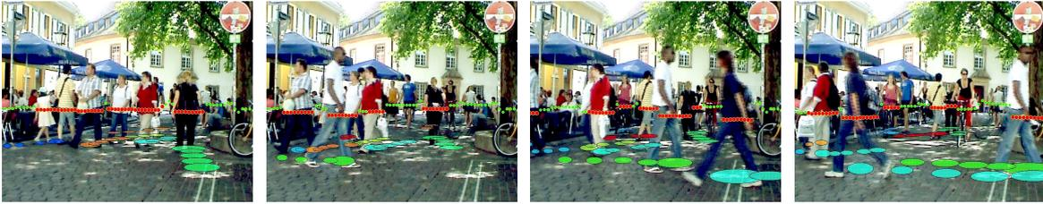
Figure 4.8: Four images of the outdoor experiments carried out in the city center of Freiburg. The information of the laser range finder and the tracking system are projected onto a recorded video sequence. The images from left to right show the tracking results at timesteps  $t = 335, 353, 365$  and  $381$ . Laser range measurements are shown as small green dots (background) or small red dots (detected pedestrians). The traces of the observed pedestrians are drawn with colored ellipses.
