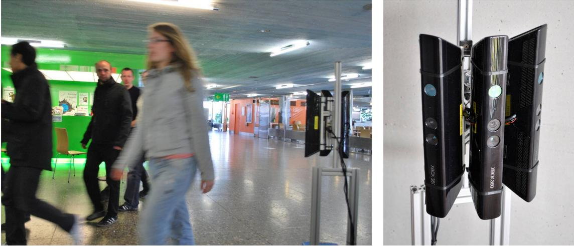
Figure 9.10: The setup consisting in three vertically mounted Kinect sensors offering a joint field of view of  $130^\circ \times 50^\circ$  and supplying RGB-D data with a resolution of  $1440 \times 640$  pixels at  $30 \text{ Hz}$ . They are mounted at  $1.2 \text{ m}$  height.
