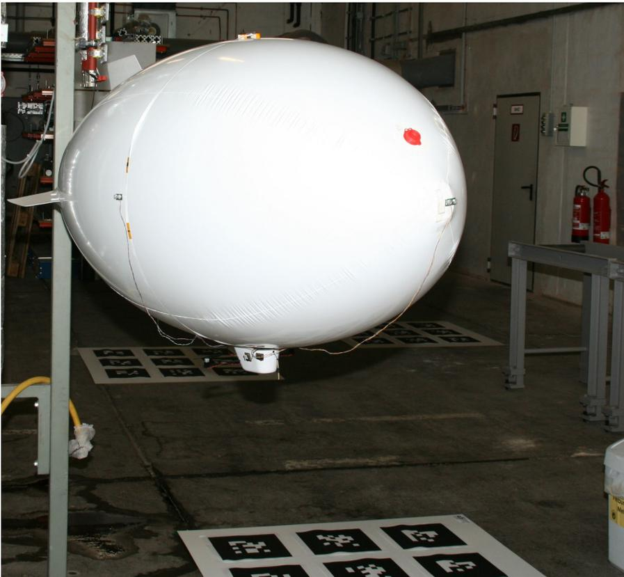
**Figure 2.9:** Our first prototype of the blimp in the experimental environment. The reference poses are obtained using the camera integrated in the gondola pointing downwards and observing the visual markers placed on the floor.
