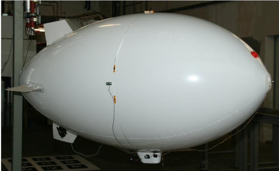
**Figure 2.1:** Our first prototype of the robotic blimp. It is equipped with three sonar sensors at the front, left, and right side of the hull as well as a sonar sensor integrated in the gondola pointing downwards. The IMU is placed on top of the hull.
