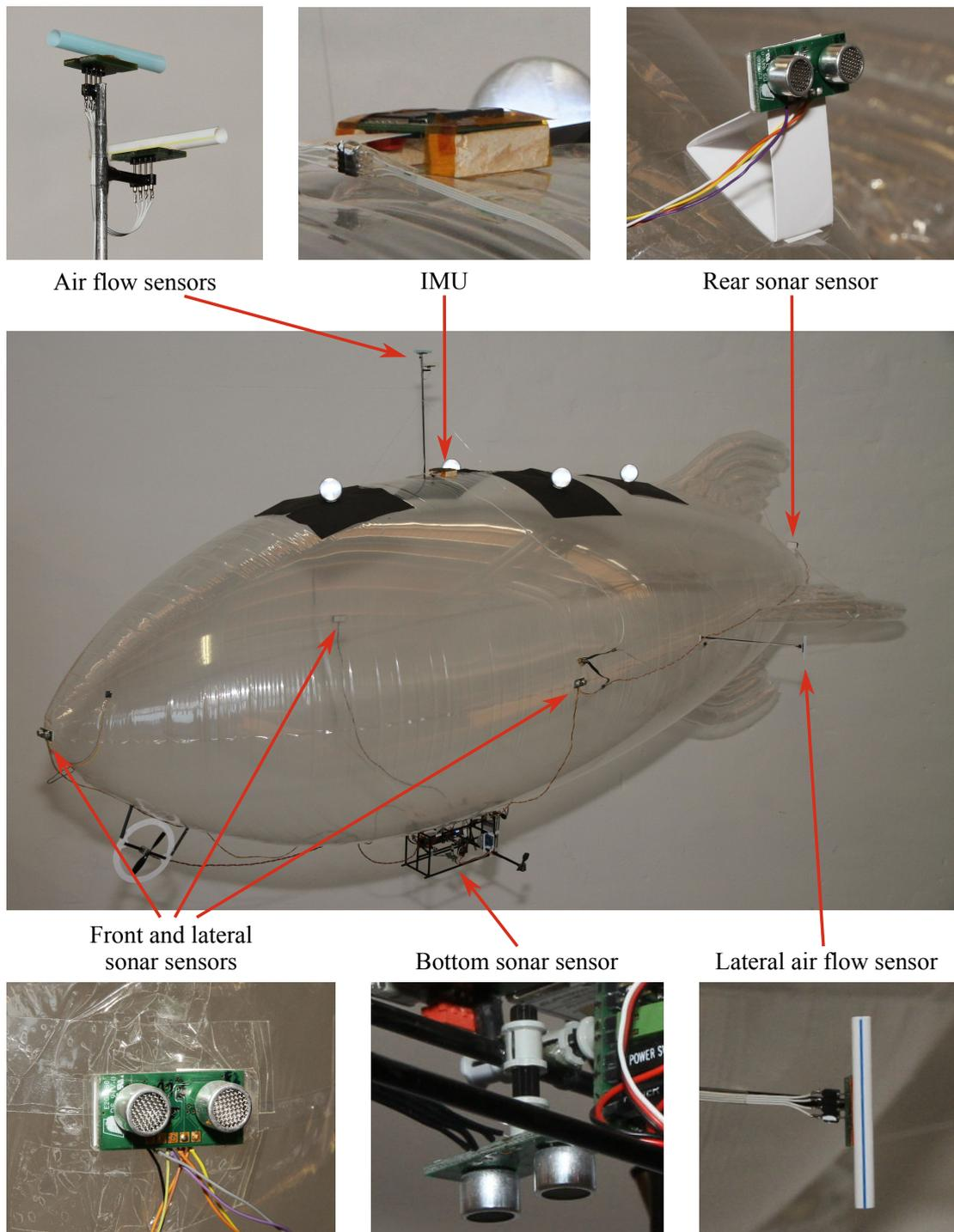
**Figure 2.3:** Our third prototype of the robotic blimp. It is equipped with four sonar sensors at the front, back, left, and right side of the hull. The fifth sonar sensor is pointing downwards and integrated in the new gondola, which provides a lightweight, modular, and easily accessible frame for the electric devices. The IMU is placed on the top of the hull. Three air flow sensors are mounted on poles for velocity measurements along all three axes.
