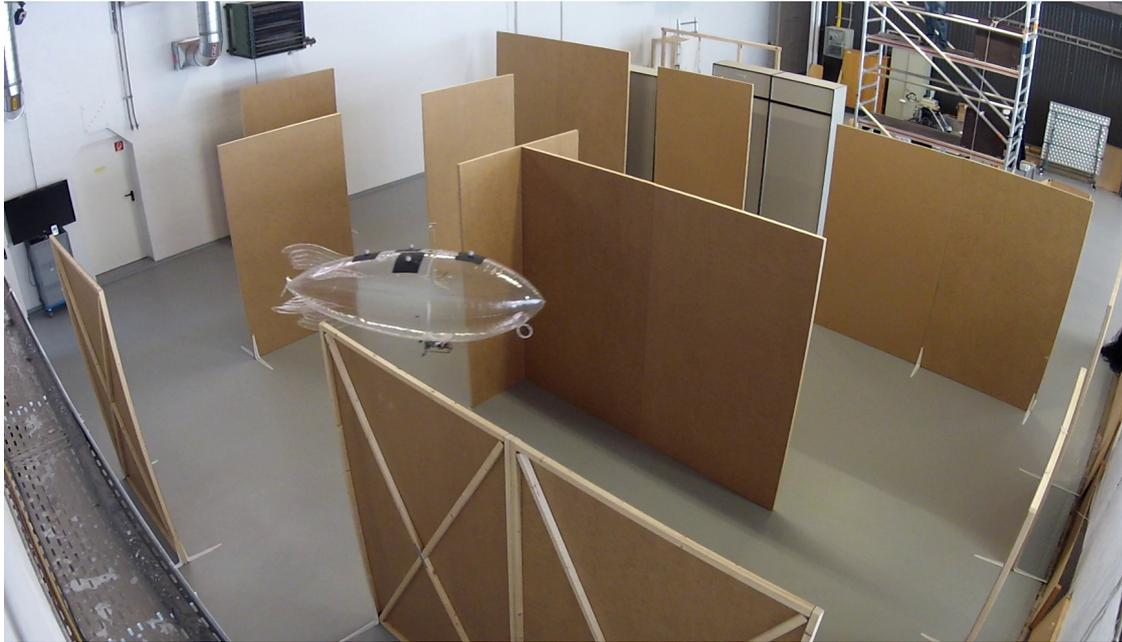
**Figure 6.1:** The third prototype of our miniature blimp operating in the maze-like indoor environment.
