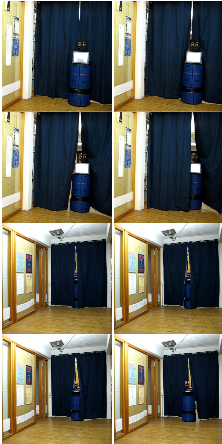
Figure 6.18: The mobile robot Albert is navigating through curtains. The first four snapshots show the robot approaching the curtains and the last four snapshots show the robot passing through from the other side of the corridor.
