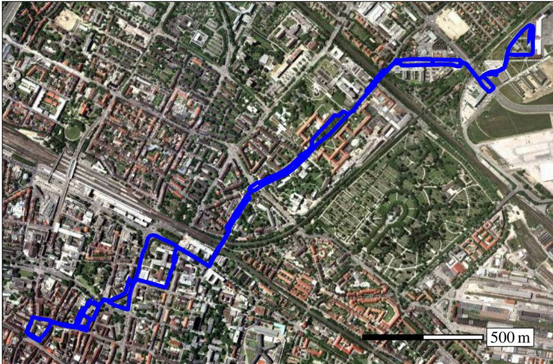
**Figure 9.9:** The pose-graph of the map used for the experiments on top of an aerial image. The trajectory as it is estimated by our approach aligns well with the aerial image (aerial image © Google).
