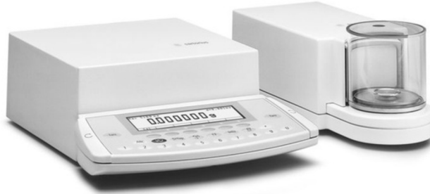
Figure 2.1 High precision balance - Sartorius SE 2 [26].
