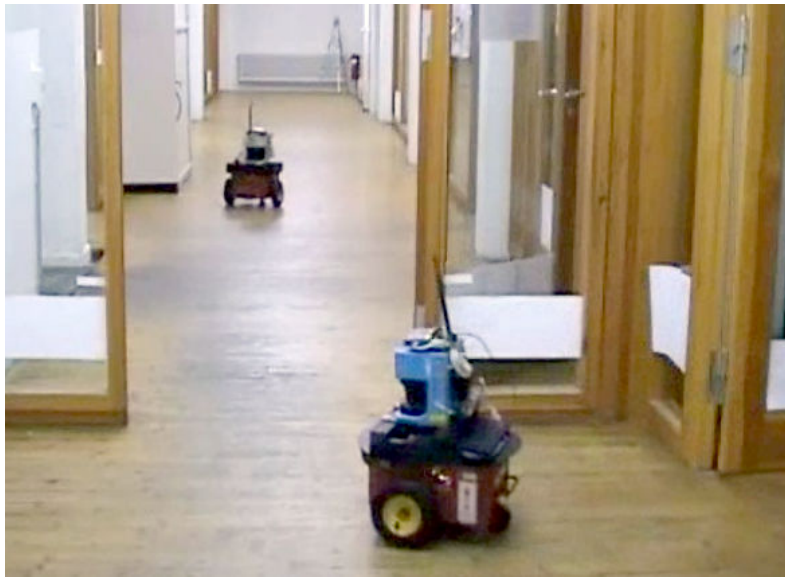
Figure 2.9: Two Pioneer II robots exploring the AIS laboratory of the University of Freiburg using our segmentation-based coordination approach.
