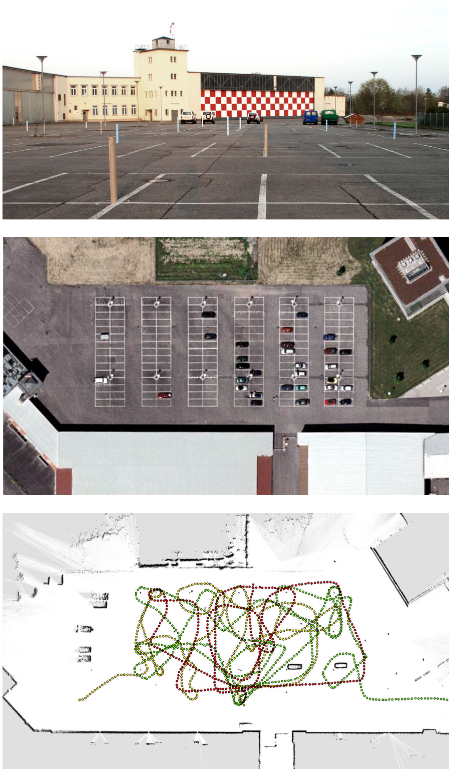
Figure 4.13: Parking lot with landmarks (top), an aerial view of the parking lot (middle), and grid map of the environment with overlaid trajectories (bottom left). Aerial image courtesy of Google Maps, Copyright 2008, DigitalGlobe.
