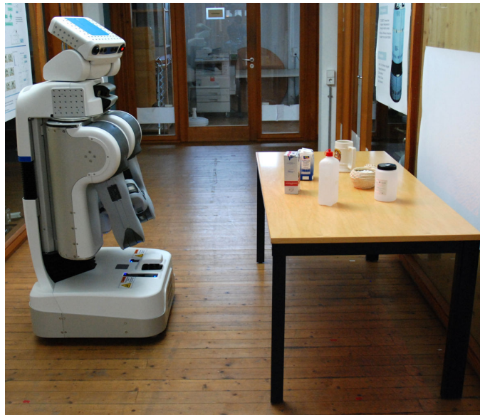
Figure 5.18: Experimental setup. A PR2 robot measures objects on a table using its stereo camera.
