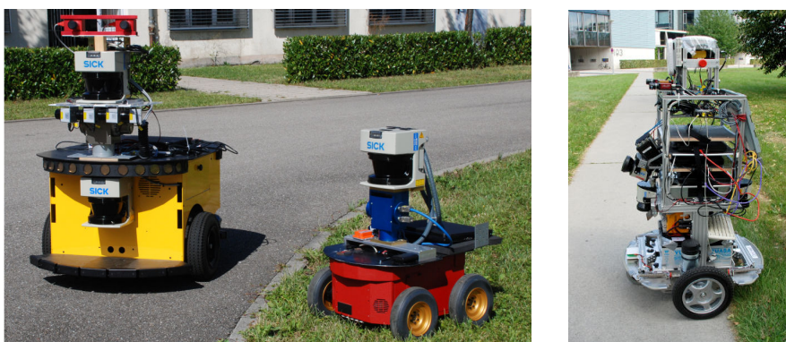
Figure 6.13: Robots used in our experiments. Left: An an ActivMedia PowerBot (yellow) and an ActivMedia Pioneer 2 AT (red), both equipped with SICK LMS 291 laser range finders. Right: The EUROPA platform equipped with a SICK LMS 151 sensor.
