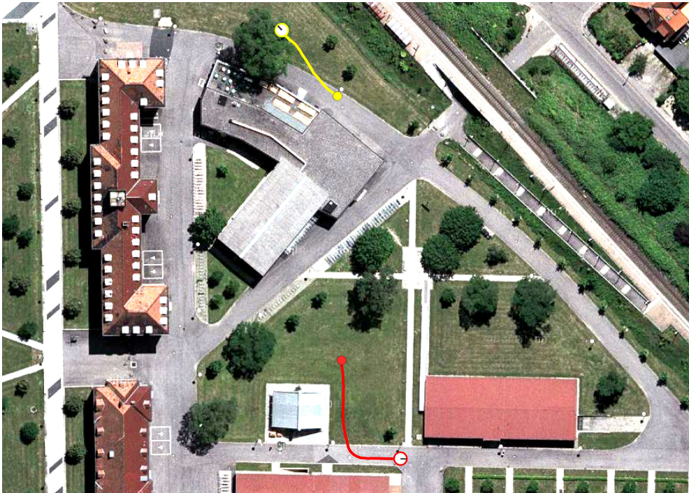
Figure 6.15: Aerial view of the computer science campus in Freiburg. Estimated robot trajectories are shown for the training (top, yellow) and the test set (bottom, red). Aerial image courtesy of Google Maps, Copyright 2008, DigitalGlobe.
