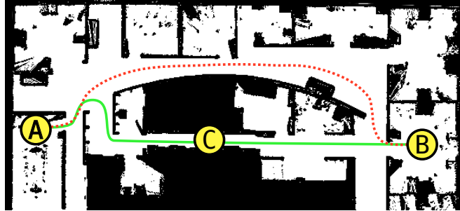
Figure 4.9: Experimental setup for the path planning experiment. The task consists in navigating between A and B . At C we added a virtual door that changed its state over time.
