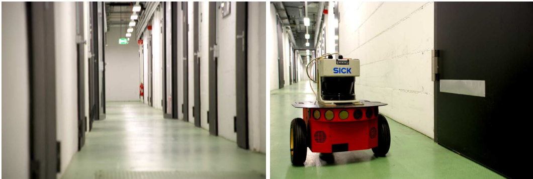
Figure 5.6: The building 103 of Department of Computer Science at the University of Freiburg consisted on a long, featureless corridor of approximately 80 \times 3 meters size. Data was gathered using a MobileRobots Pioneer P3-DX robot equipped with a SICK LMS 291 laser range finder. As landmarks (right image), stripes of retro-reflective material were taped to the walls in the locations indicated by our approach.
