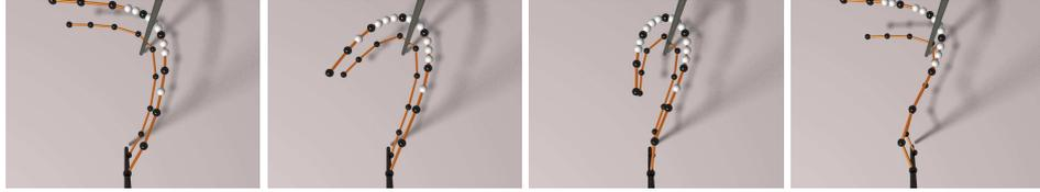
Figure 4.3: Two rods with equal material properties are colliding with a rigid obstacle. One rod is dynamically refined while the other rod has a fixed resolution. The four images illustrate that the dynamic behavior is not affected by the refinement.
