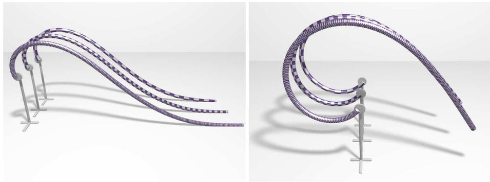
Figure 3.12: Coiling up three clamped rods. The rods are discretized into 1000, 100 and 50 elements, illustrating that the global deformation is independent of the discretization.
