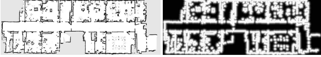
Figure 3.3: Occupancy grid map (left) and likelihood field (right) of the ground floor of building 079 at the University of Freiburg.
