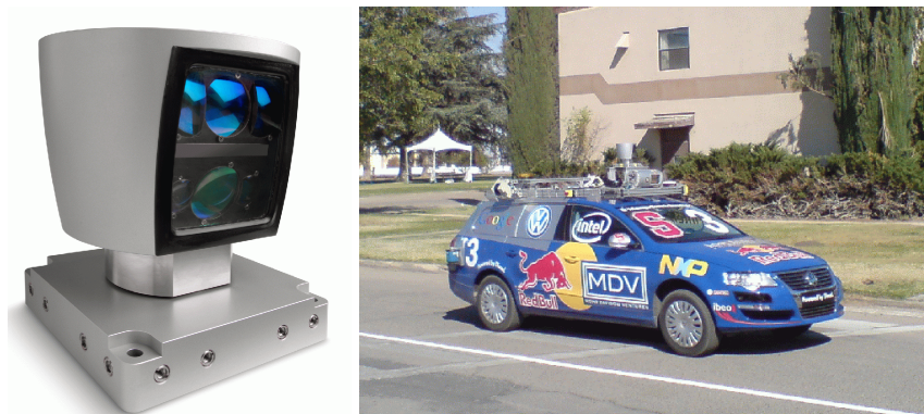
Figure 11.2: Velodyne HDL-64E Laser Sensor used for 3D-mapping (left) which is mounted on the robot car named Junior (right).
