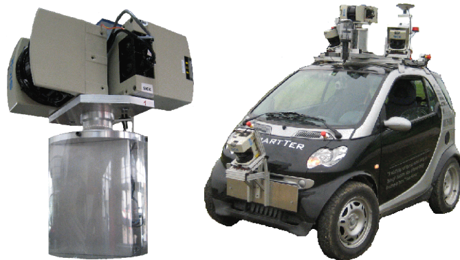
Figure 11.1: Two vertically mounted SICK LMS laser range finders (left) which are rotated with constant speed by an electric step motor mounted under the lasers. The right image shows our robot. The robot is a standard Smart car (right). The model is a Smart fortwo coupé passion of the year 2005, which is equipped with a 45 kW engine.
