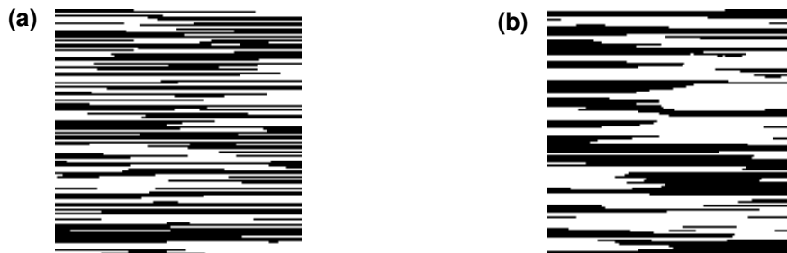
Figure 4.5: Typical images simulated by the Gibbs sampler using the anisotropic auto-logistic potential function in Equation (4.4) with \beta_h = -10 , \beta_v = 0 and \alpha = 10 in image (a) and \beta_v = -0.1 and \alpha = 10.1 in image (b).
