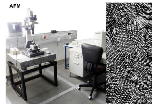
Fig. 1: AFM: MultiMode AFM Nanoscope IIIa, Veeco
