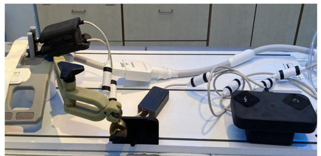
**FIGURE 2.** The experimental setup for phantom targeting. The instrument positioning unit (IPU) is positioned over the target region using a dedicated MR-conditional flexible holding arm.
