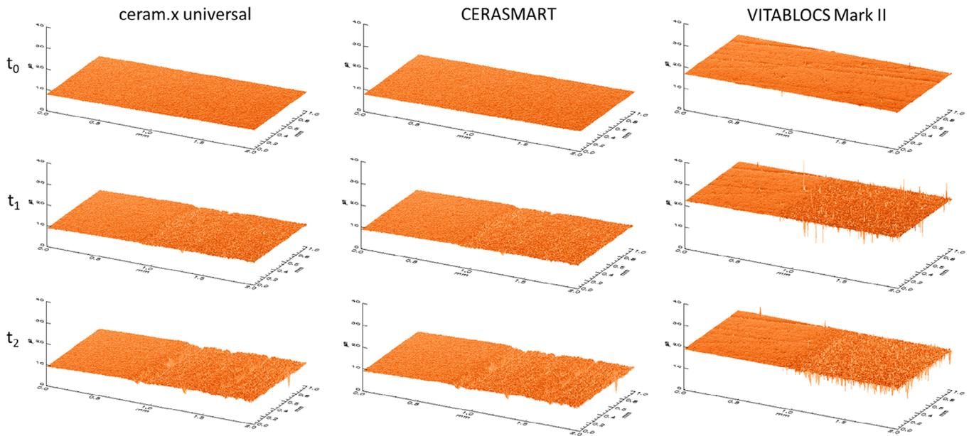
**FIGURE 6** Exemplary images of 3D profilometric data of materials ceram.x universal, CERASMART and VITABLOCS Mark II at baseline ( $t_0$ ), at 12 months ( $t_1$ ), and at 36 months ( $t_2$ ).
