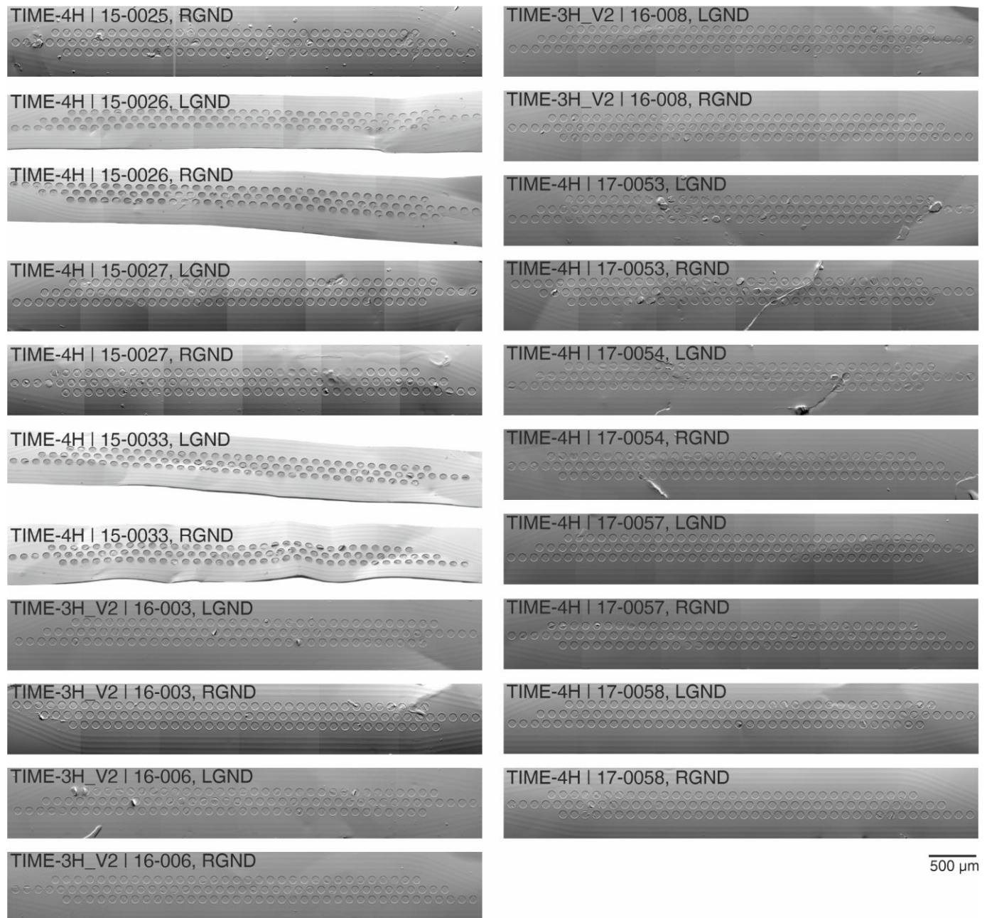
Supplementary Figure 2. Overview of all explanted and available ground contact sites for optical analysis. Images were acquired with SEM.
