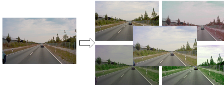
Fig. 3.8 A2D2 Pool-Aug. Left: the original image. Right: the duplication through color augmentation and random cropping of the original image
