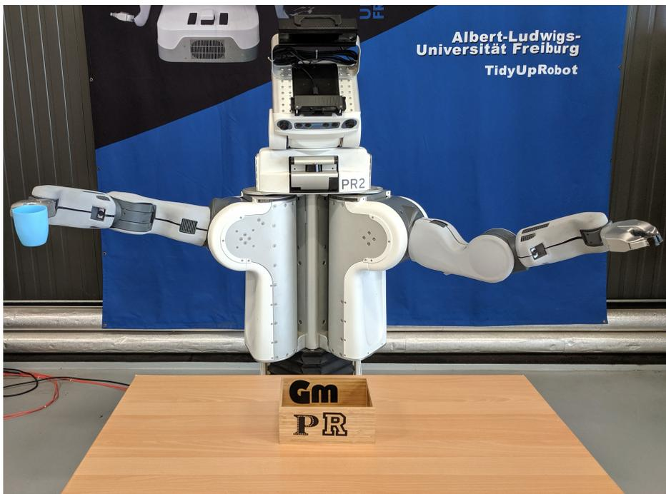
**Figure 1.1:** The PR2 mobile manipulation robot that we use in our experiments. The robot has two arms and a mounted Kinect 2 RGB-D camera on its head.
