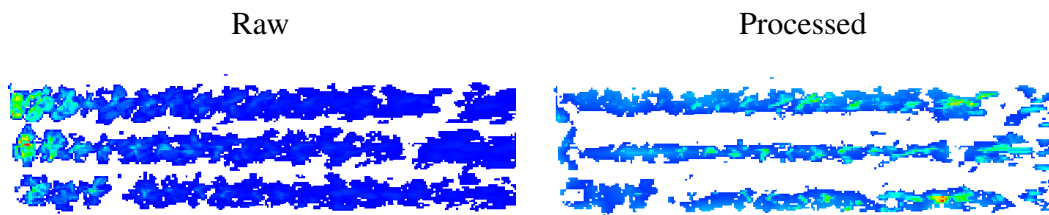
Figure 2.2: On the left, a portion of the raw feature map obtained by applying the triangular greenness index on an image is shown. On the right, we show the feature map after processing by weighting each point with its squared distance to the camera, applying a lower bound and smoothing the weights. The color scheme is a heat map on the rainbow spectrum, where blue corresponds to low feature weights, and red corresponds to high feature weights. The white space has feature weight 0.
