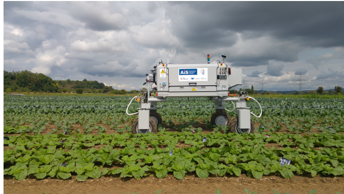
Figure 1.1: This picture shows our agricultural robot BoniRob on a production vegetable field. It has a high ground clearance and is able to adjust its wheel positions by changing the angles of the lever arms to which the wheels are attached. We use it as an experiment platform to test our approaches in real world scenarios.
