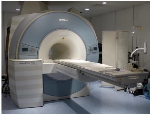
Figure 5.4: 3 T whole-body MRI system (Tim Trio, Siemens, Erlangen, Germany) used in the FMISO trial.
