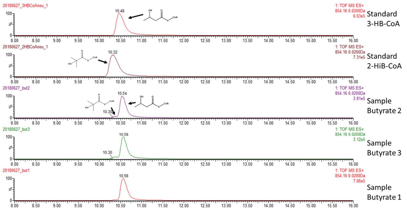
**Fig. S1 HPLC-MS chromatograms from lysates of acetone (Sample Acetone 1-3)- and butyrate (Sample Butyrate 1-3)-grown cells compared to pure standards of 2-hydroxyisobutyryl-CoA (2-HiB-CoA) and 3-hydroxybutyryl-CoA (3-HB-CoA).** Acetone-grown cells show substantially more 2-hydroxyisobutyryl-CoA (elutes between 10.30 - 10.45 min) whereas in butyrate-grown cells mainly 3-hydroxybutyryl-CoA (elutes between 10.48 - 10.58 min) was identified.
