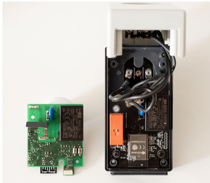
Figure 4.8: Two versions of the PowerMeter hardware. Initial plain PCB (left) with a serial connector and second iteration (right) with a modular expansion header and primed for continuous wireless data streaming.
