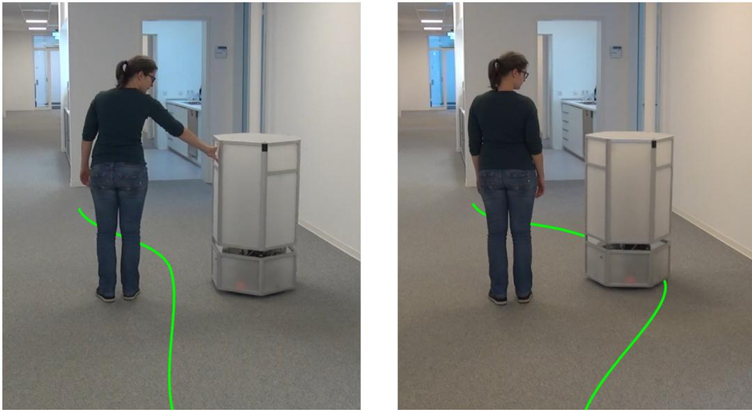
**Figure 5.1:** A person communicates her personal space preference by pushing the navigating robot away from her (left). Based on this interaction, the robot adapts its navigation behavior and learns to keep a greater distance to people (right).
