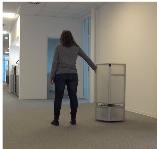
**Figure 5.6:** Participants guide the navigating robot past themselves with the joystick (left) and force feedback (right).
