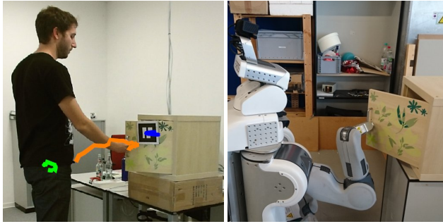
Figure 4.8: Demonstration and robot execution. On the left image the teacher demonstrates the task of opening the swivel door. Superimposed on the image the recorded trajectories for hand (orange), torso (green) and manipulated object (blue) are shown which serve as the input for the action learning. The right image shows the robot reproducing the action using a model learned from the teacher demonstration.
