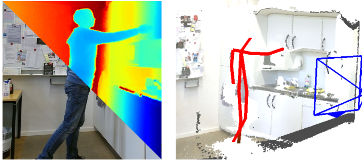
Figure 4.1: Problem overview. Given a color image and depth map, our system detects body keypoints in 3D, which are useful for many robotic tasks. Exemplary use in a learning from demonstration setting was described in detail in the respective paper [152] and is shortly summarized in Section 4.6.3.
