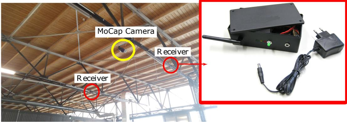
**Figure 3.3:** Sender localization system (ASSIST). The speaker of an out-of-the-box smartphone is used as a sender. [7]
