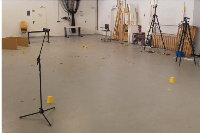
**Figure 8.4:** A smartphone was placed at eight different positions. Four of them with a height of 1.39 m and four of them with a height of 2.12 m. [7]
