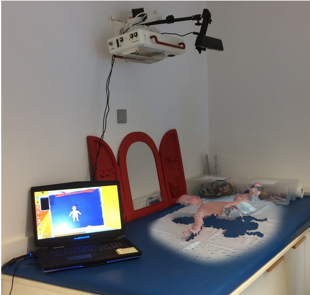
Figure 3.1.: Recording setup. RGB-D camera mounted 1 m above examination table, facing down. Connected to laptop. Scene overlaid with infant point cloud.
