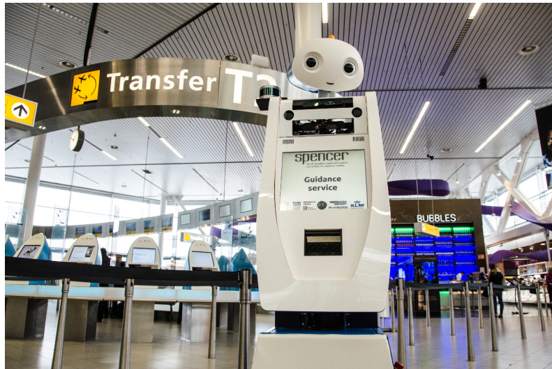
Figure 8.2: The Spencer robot at Schiphol. The robot has a screen to interact with the passengers. A boarding pass scanner, located under the screen reads the passengers' gate information. Once the robot has read this information, it guides the passengers to their gate of departure.
