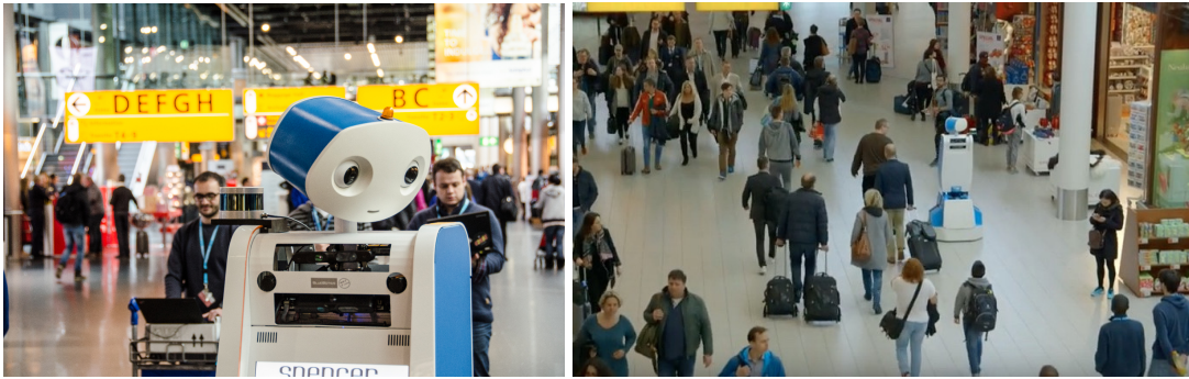
Figure 8.15: The Spencer robot while testing its navigation capabilities at Schiphol.
