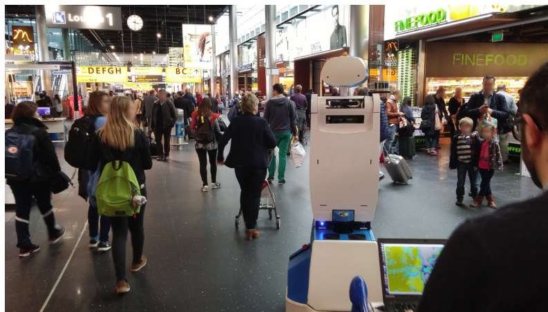
Figure 8.4: The robot faces a crowd at Schiphol, the environment is densely populated and highly dynamic, it has no free ways to the goal. The robot risks to be "frozen", to be trapped into the crowd.
