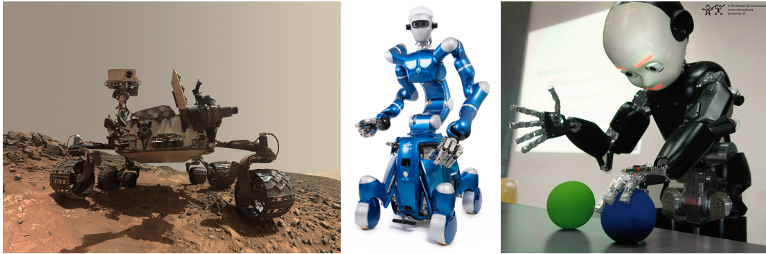
Figure 1.1: Example robot applications. Left: Curiosity is a Mars rover created by the NASA who drove autonomously on Mars 14.14 km as of 8 September 2016. Center: The Rolling Justin robot an advanced mobile dual-arm system developed by DLR. Right: ICub robot designed by the Italian Institute of Technology, a robot that has not only manipulation capabilities but it is able to express emotions by using its facial expressions.
