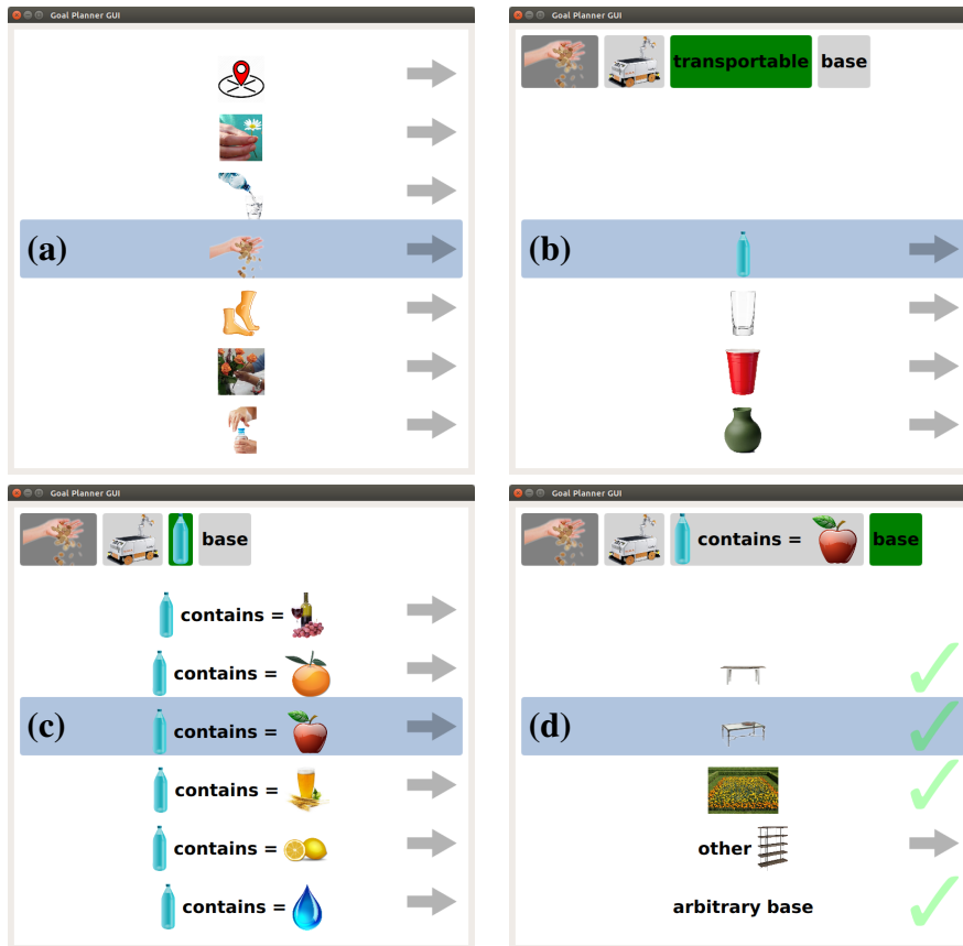
Figure 6.4: Graphical user interface of the high-level planner. (a) Selection of a high-level planner action. (b) Refinement of the action parameter of type transportable . (c) Refinement of the argument based on content . (d) Refinement of the last action parameter of type base .
