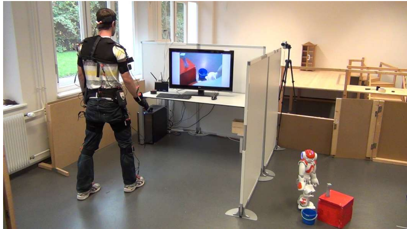
Figure 2.12: Teleoperation with visual feedback. Left: Human operator and live view of the robot’s camera displayed on a monitor. Right: Teleoperated Nao humanoid.
