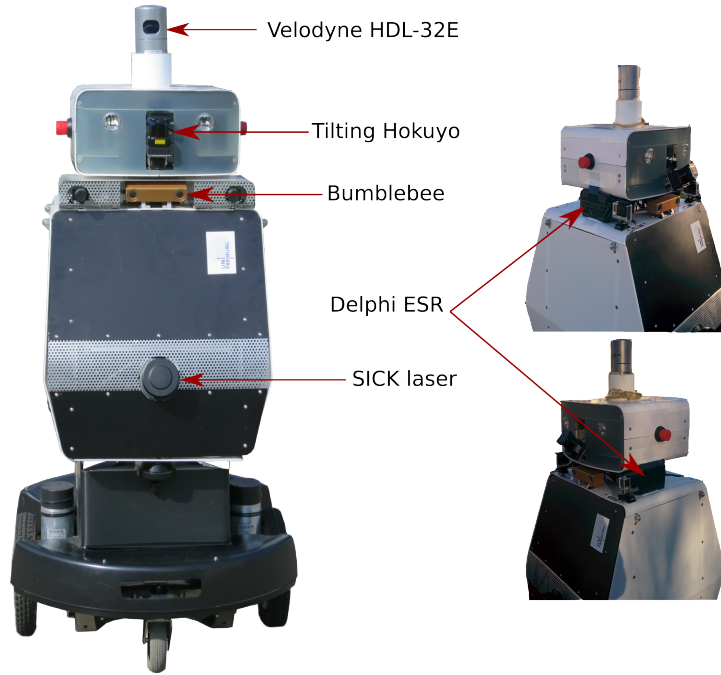
Figure 2.1: Our robotic platform (Obelix) that was used for capturing the different datasets and conducting real-world experiments.
