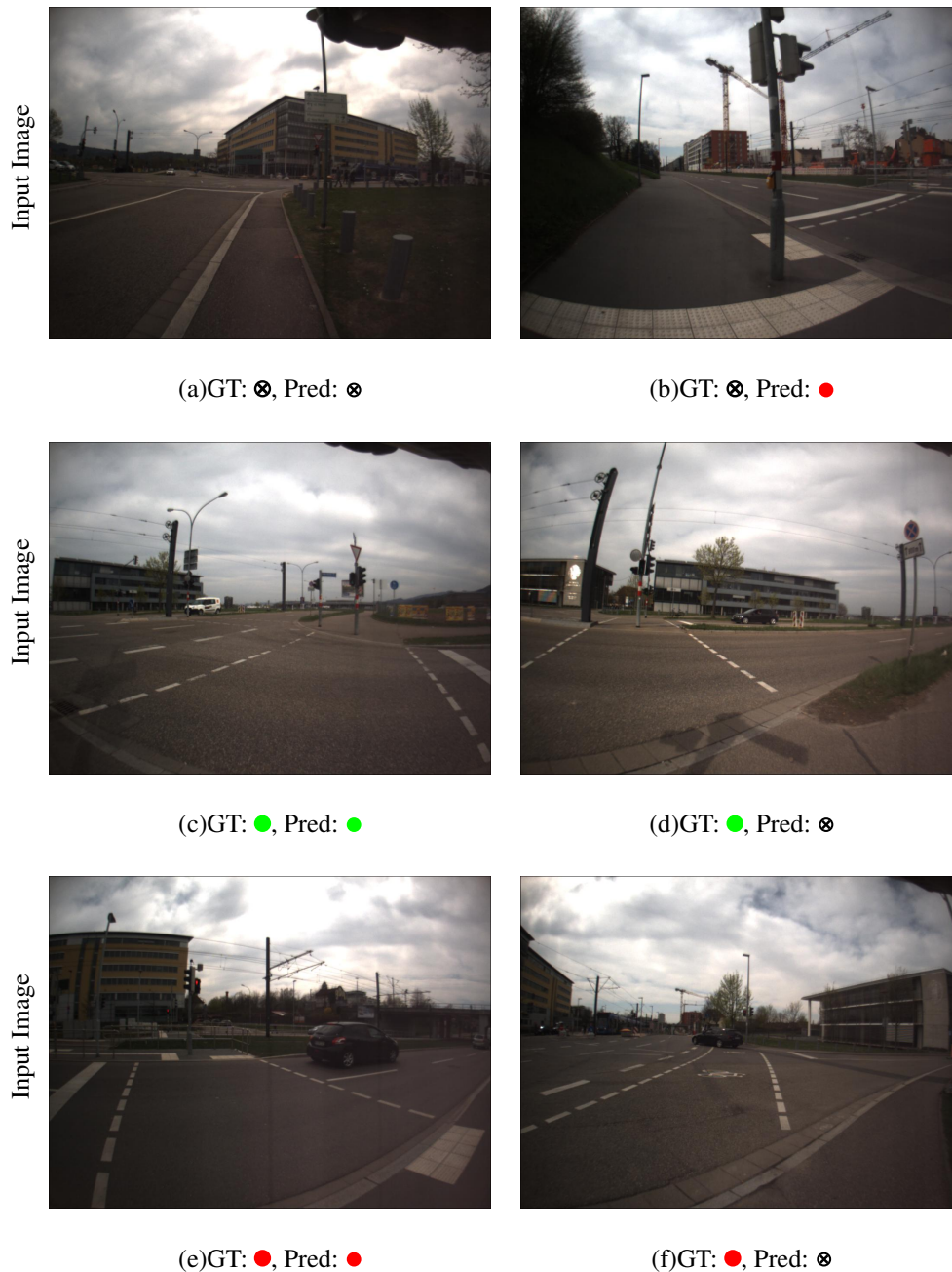
Figure 5.14: Qualitative analysis of the proposed traffic light recognition method on the Freiburg Street Crossing (FSC) dataset. Figures (a, c, e) illustrate correctly predicted images, while figures (b, d, f) illustrate mispredicted images. The small size of the traffic lights (fig. (c, f)), presence of noise sources (fig. (b, e)) and the varying illumination conditions (fig. (a, d)) under which the dataset was captured adds to the difficulty of the dataset for the given task. Despite these challenges, our approach is able to accurately recognize the state of the traffic light (fig. (a, c, e)).
