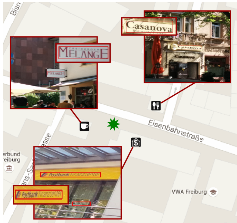
Figure 3.1: Overview of our text-based localization approach: Standing at a certain position, we capture images of the neighboring shops. Using text spotting, we extract the text information to match the observation with geo-referenced texts from the map and generate a pose estimate.
