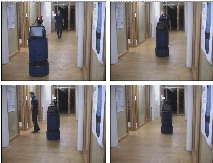
Figure 4.12: Albert moves forward and waits until the likelihood of interfering with the person is low enough.
