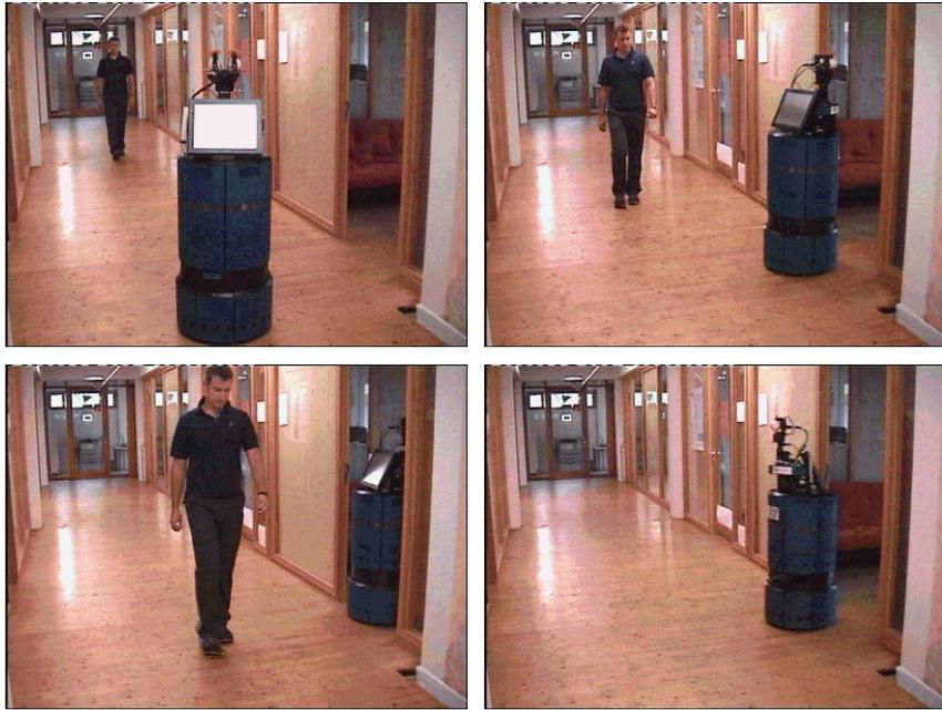
Figure 4.6: To avoid that the person has to slow down Albert moves into the doorway and continues its way after the person had passed by.
