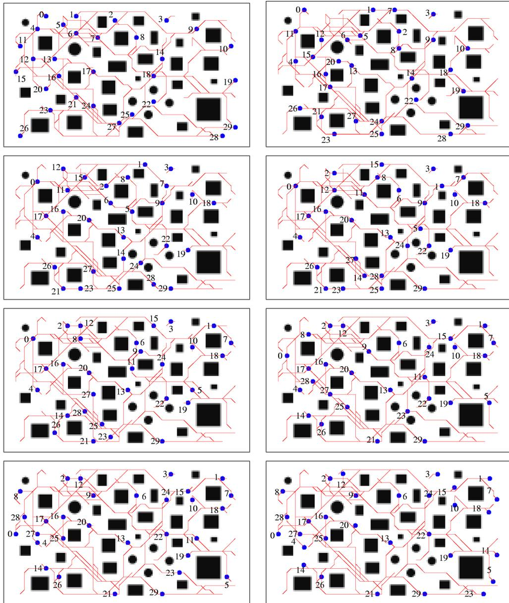
Figure 2.22: This figure shows images of a simulation run in which the robots carry out the paths of the best solution which was found. The upper left image shows the robots at their initial position, the upper right images shows the position of the robots at time step 9, the left image in the second row at time step 17 and so on. In the situation depicted in the image in the lower right all robots have arrived at their goal position.
