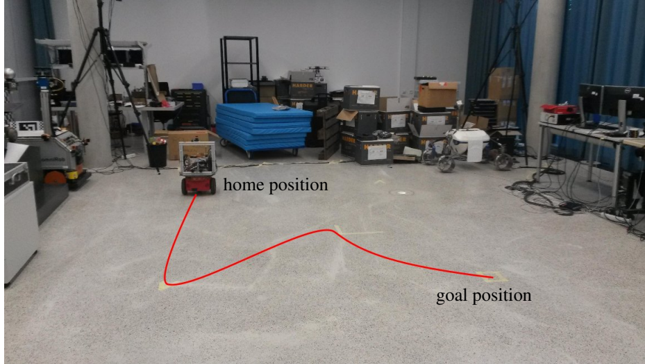
Figure 3.44.: Experimental setup for the indoor laboratory experiment with home position, path and goal position
