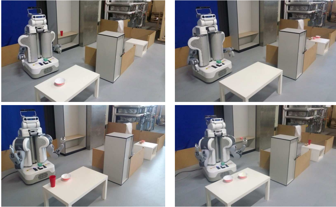
Figure 5.5: This figure shows four of the evaluation settings. The task was to bring all objects to the front table and wipe the spot under each object.
