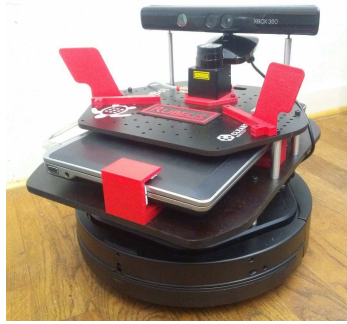
Figure 6.9: One of the Turtlebot 2 robots used in the experiments with a Kinect sensor and Hokuyo laser.
