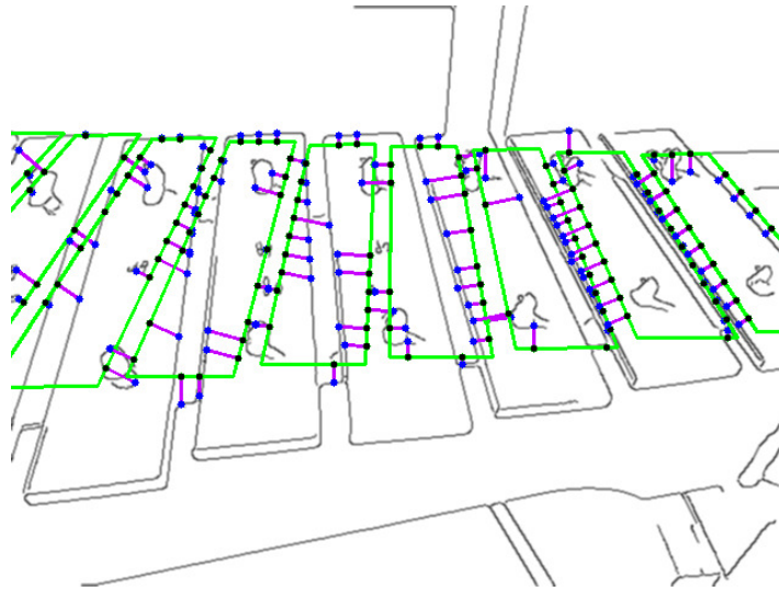
Figure 6.3: Example for likelihood computation in instrument tracking. Green lines are the model edges according to a pose hypothesis, with sampled points (black dots). Gray indicates canny edges, blue dots are detected matches to the green dots. The magenta lines indicate the residuals used in the likelihood computation. Only successful matches smaller than a maximum distance are shown.
