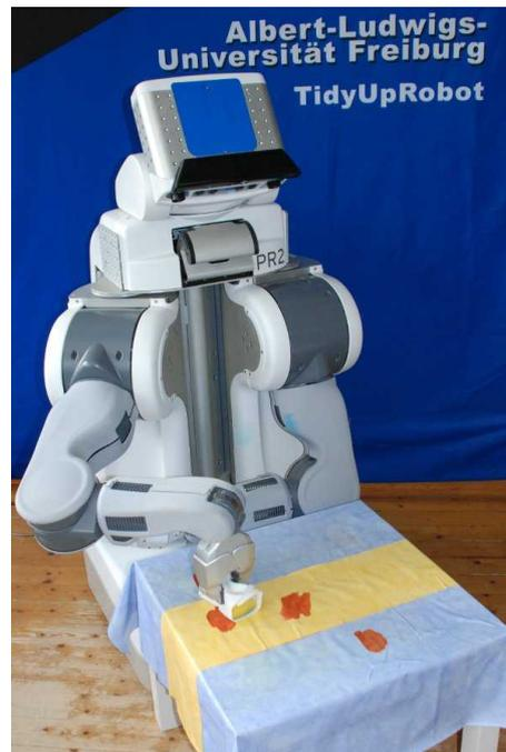
**Figure 5.1.:** PR2 robot using a sponge to remove dirt (seen in brown) from a table. Instead of cleaning the whole table, the robot observes the outcome of its actions, learns which features correspond to dirt, and cleans only the dirty regions.
