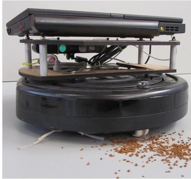
**Figure 6.1.:** Roomba 560 robot used in the experiments. The vacuum cleaning unit of the robot is equipped with a dirt detection sensor. The mounted Asus Xtion Pro Live depth camera is used for localization.
