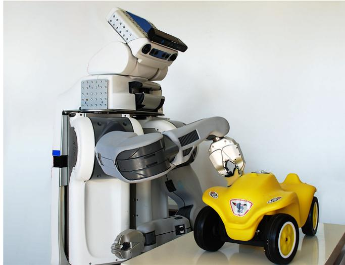
**Figure 4.1.:** PR2 robot using a sponge to clean a toy car.
