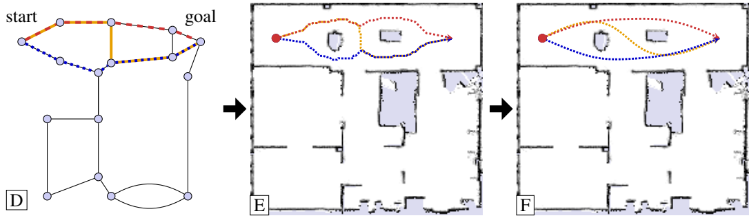
Figure 4.6: Computing the k best paths from the Voronoi diagram. (D) Graph representation of the Voronoi diagram. Each path in this graph corresponds to a homotopically distinct path from start to goal. (E) Trajectories generated from the three shortest paths. (F) Optimized trajectories.
