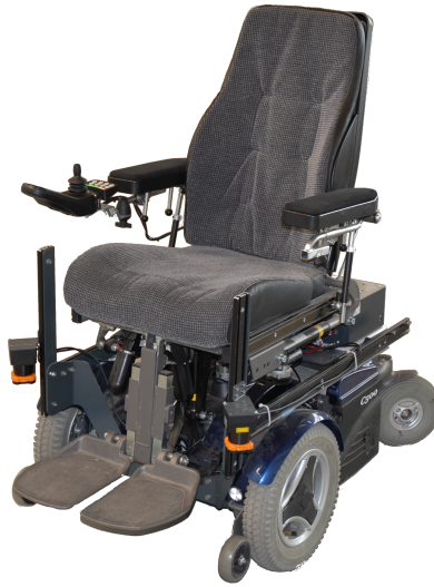
Figure 5.9: Autonomous wheelchair used for the experiments. We equipped the Permobil C500 wheelchair with wheel encoders, two laser range finders at the front and a control interface to send joystick commands to the wheelchair. For processing the navigation algorithms, we mounted a small desktop computer at the back of the wheelchair.
